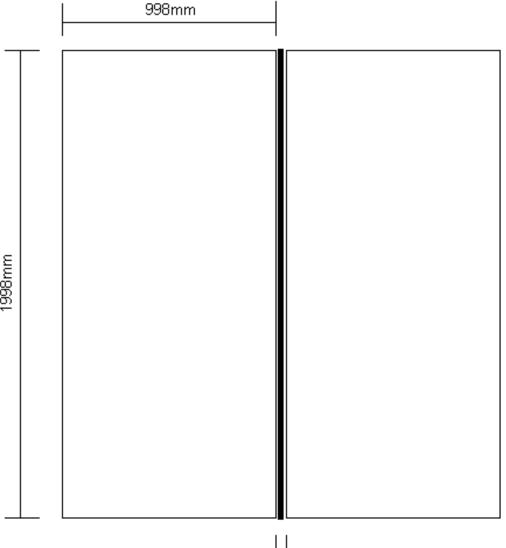
The image shows a 2m wall section in our panel and pole system.
